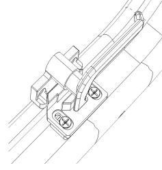
When installing the catchers take care to align the catcher with the groove on the handle.
